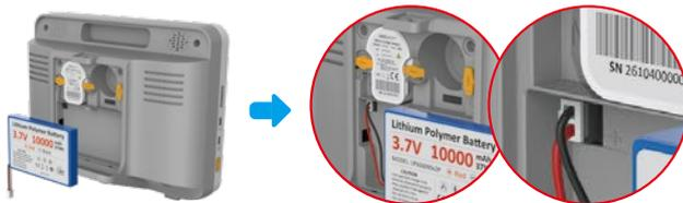
Open the back cover of the instrument, insert the battery connector plug into the battery connector socket in the direction indicated by the positive and negative poles (red for positive, black for negative) and then place the battery into the battery compartment.
