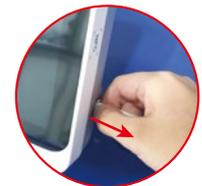
**Disassembly:** Press and hold the ring on the instrument, then remove the air tube.
